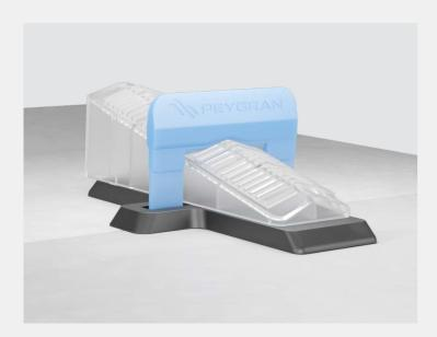
Wedge-bases have been made to extend the functionalities of our system allowing us to work with thicknesses from 3 to 5mm. Use it in thicknesses lower than 5 mm and in thicknesses from 16 to 20mm. Place the clips under the wedge, allowing the wedge to be centered and providing a larger support surface.
