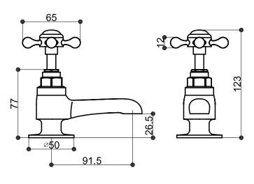
Identify the hot tap and position into the basin on the left hand side, from the underside of the basin fit the rubber washer and then the nut. Making sure the tap is in the right position tighten the nut to secure the tap to the basin.
