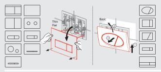
2. Remove the complete flush plate from the concealed cistern. First of all release the locks used to fasten the flush plate frame. Then use the side clamps to release the flush plate itself and remove it.
