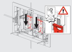
4. Put the flush plate back, check the compression clearance – it should be 1–2 mm.
