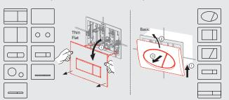
Set the appropriate distance of the screws that are used to adjust the correct clearance of each button. Use the cartoon template that you will find in the package of your flush plate.
