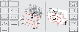
2. Remove the complete flush plate from the concealed cistern. First of all release the locks used to fasten the flush plate frame. Then use the side clamps to release the flush plate itself and remove it.
