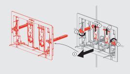
3 Remove the inner plate separating the flush plate from the concealed cistern. You can remove the inner plate by clicking out the grips on the upper edge of the plate.
