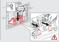
Check the functionality of the small flush lock. When the small flush button is pressed, the lock must swing to the left and hit the center reinforcement.
