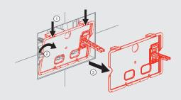
5. Check that the flushing mechanism is properly placed in the cistern and is securely fastened. The mechanism must fit into the two openings on the rear wall of the cistern. You should hear a click when it is inserted into the front part of the cistern. Check the correct fitting of the flush valve rod in the flushing mechanism. Once the mechanism is properly placed, attach the flushing mechanism rod from the fill valve.
