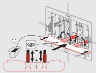
3 Checking the screw locks. Make sure that the locks used to secure the flush plate frame are locked in the bottom position, thereby fixing the position of the screws.
