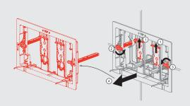
3 Remove the inner plate separating the flush plate from the concealed cistern. You can remove the inner plate by clicking out the grips on the upper edge of the plate.
