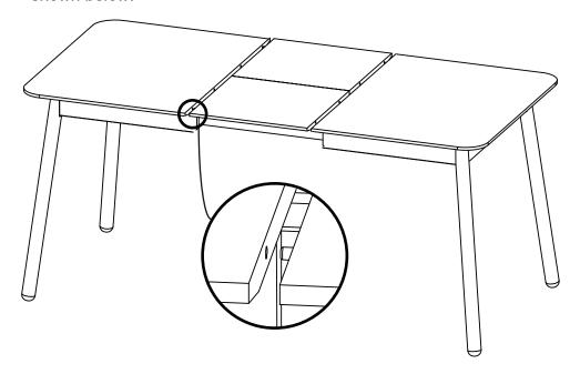
Step 6 Ensure the 2 x securing clips are fastened before using the table. To store the leaves perform this operation in reverse.
