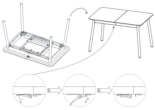
$Step\ 2\quad \hbox{{\tt Pull} end of table to oposite direction by 2 persons, open to the end position}.$
