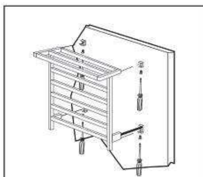
STEP7 Fix on the wall
