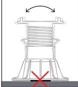
The bottom sheet fits perfectly to the base for vertical closing. In this way, the entire base of the Pedestal is supported correctly and has no reduction in resistance.
