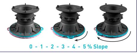
When several pieces are combined we can get all the inclination percentages lower than the maximum slope. We use several regulators to find the exact inclination. Each tab that we rotate to the regulator we add 0,25° of inclination.
