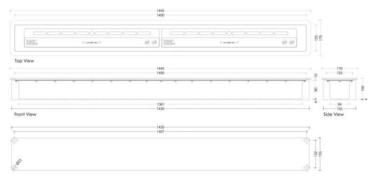
Slimline 1400 Biofuel Burner With Mount Plate
